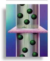
For added viral safety assurance, a nano filtration step is included, even though no human or animal components are added during the recombinant production process. **Quality Validation**
