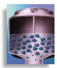
To foster cellular replication and production of rhBMP-2, they are transferred to a bioreactor, a computercontrolled, closed-system environment where large-scale production of rhBMP-2 begins. After a growth period of about three days, the recombined cells are filtered away from the rhBMP-2 containing medium and discarded. The rhBMP-2 moves on to the purification process. Purification
